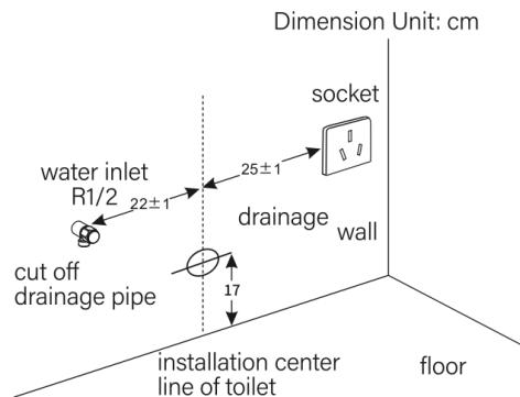
Remark: It is recommended to install water and electricity according to the dimensions shown in the diagram, otherwise it may cause the risk of pipe bending.
